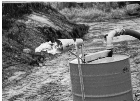
Fig. 4. Power extraction of gasoline from gravely sand during basin experiments. The vacuum pump, the collecting tank and an extraction pipe (upper). Controlled burning of gasoline vapors by the incinerator (below).
