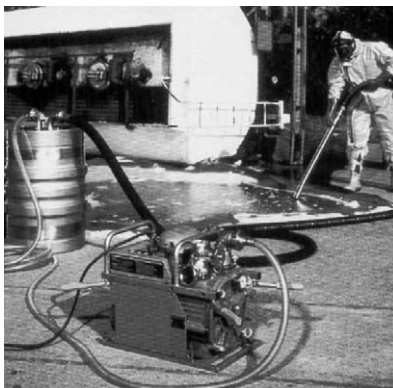
Fig. 1. Vacuum extraction based equipment for recovering spilt chemicals from liquid pools.
